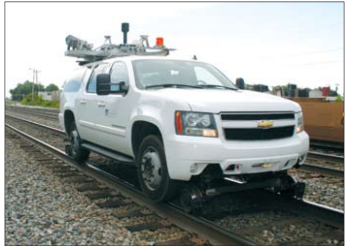
ABOVE: NCRR's Hy-rail vehicle (a Chevy Suburban equipped with rail gear) carries dual lidar sensors for one of the data collection components of the project. NCRR collected more than 300 miles of railroad centerline with this equipment.
